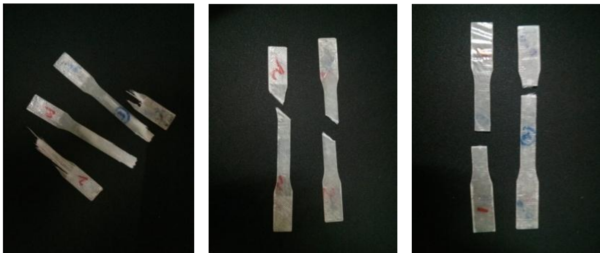
Fig 4, Fractured Test Specimens
