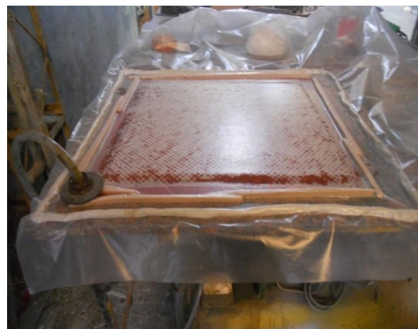
Figure 1, Manufacture of Glass fibre laminate using Vacuum hand lay – up technique
